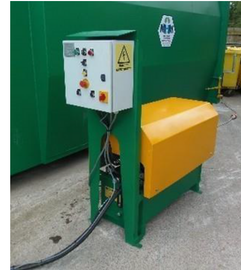
Picture Above: The stand-alone powerpack and control panel.
